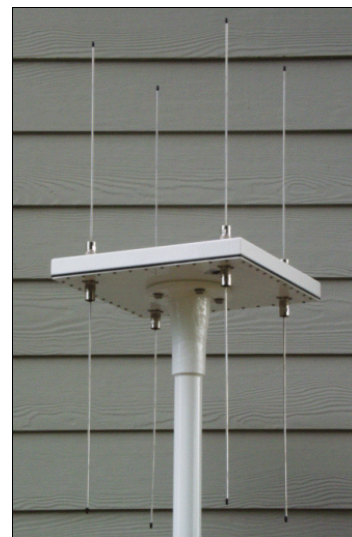
Figure 3 - Mast-Mounted H-Dipole Adcock DF Antenna
