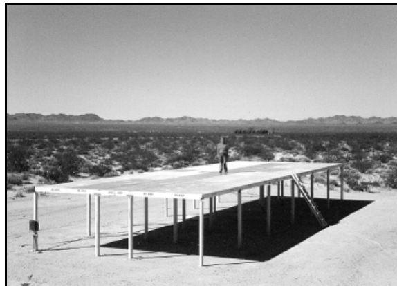
20' x 60' Elevated DF Antenna Test Range
