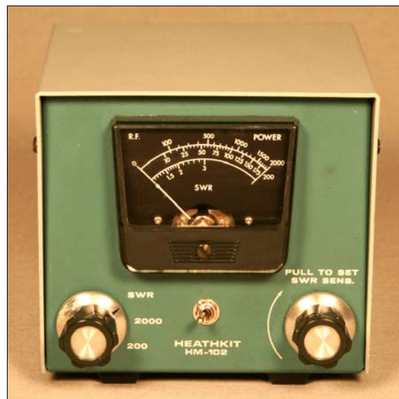
Figure 2 - Reconditioned HM-102 with Added Forward/Reflected Toggle Switch
