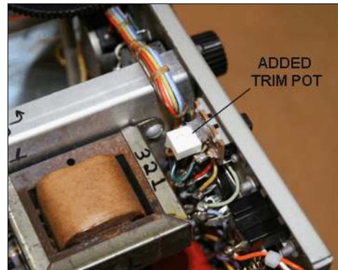
Figure 3 - Added Bias Trim Pot (mounted on H/L Bias Select switch)
