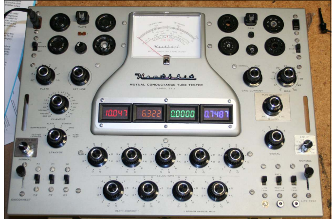
Figure 24 - TT-1B Upgrade to Numeric Displays
