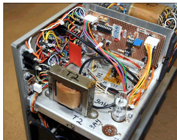
Figure 10 - Added 5.030 kHz Signal Oscillator Module
