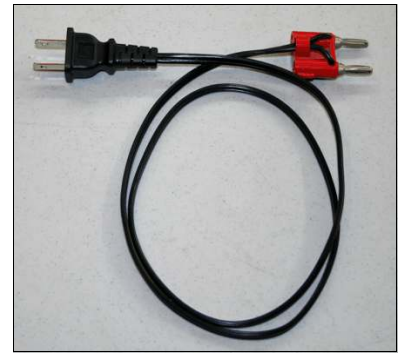
Figure 4 - Filament Voltage Voltmeter Probe
