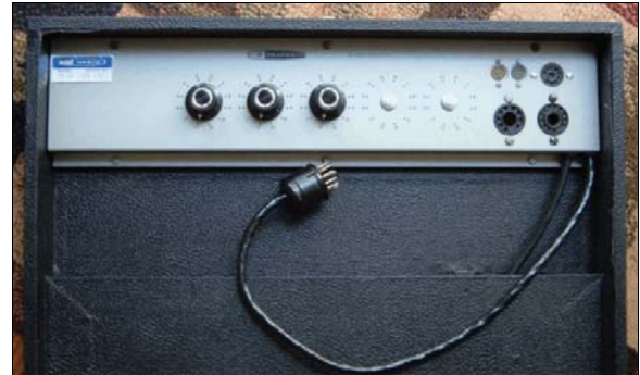
Figure 4 - TTA-1-1 Supplemental Tube Socket Adaptor Assembly (for TT-1A)
