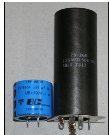
Figure 6 - Electrolytic Capacitors - Then & Now
