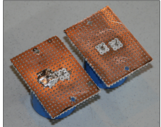
Figure 8 - Capacitor Mounts (bottom)
