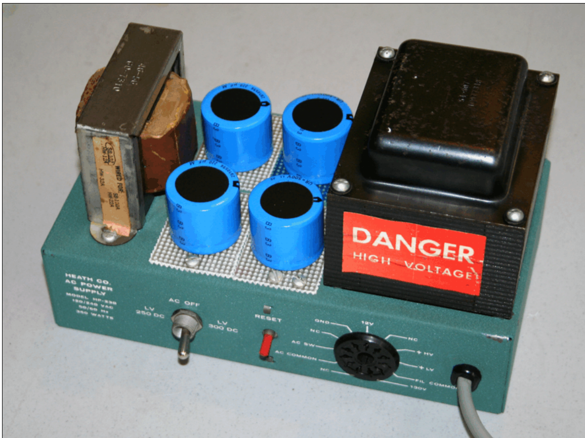
Figure 12 - Topside Photo of Fully Reconditioned HP-23B
