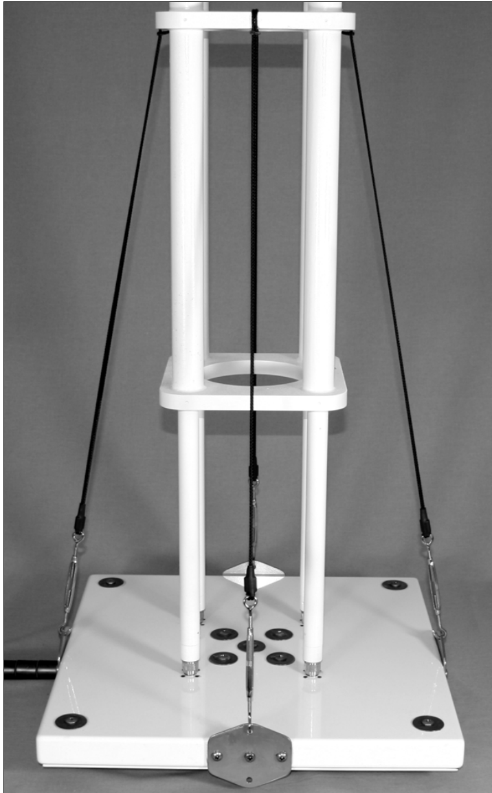
Figure 6 - Sleeve-Dipole Array Kevlar Guy Line Installation
