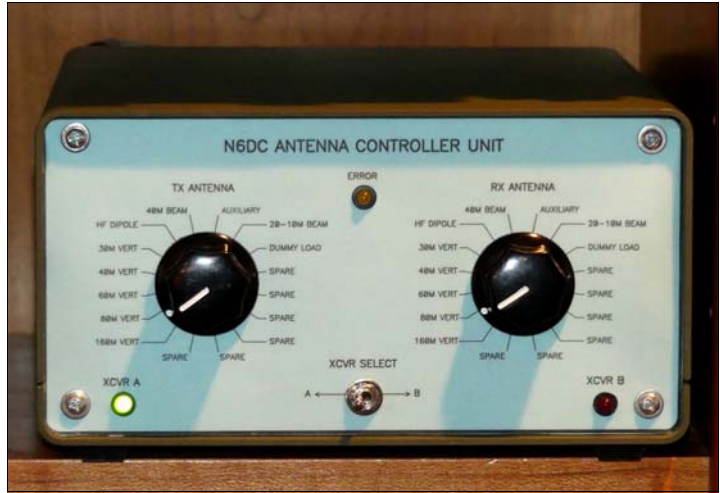
Figure 12 - N6DC Antenna Controller Unit (ACU)
