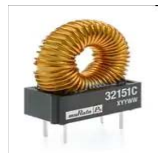
Figure 3 - Murata Toroidal Power Inductor (150 uH)
