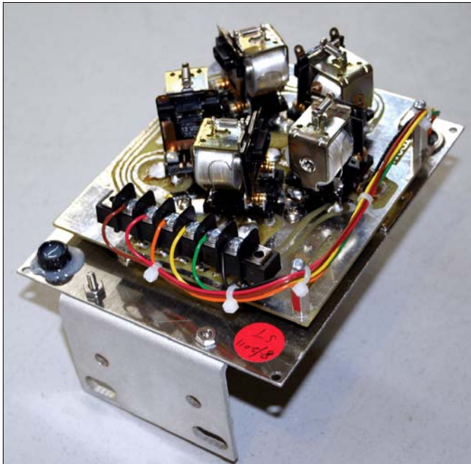
Figure 7 - Interface Connector Wire Routing
