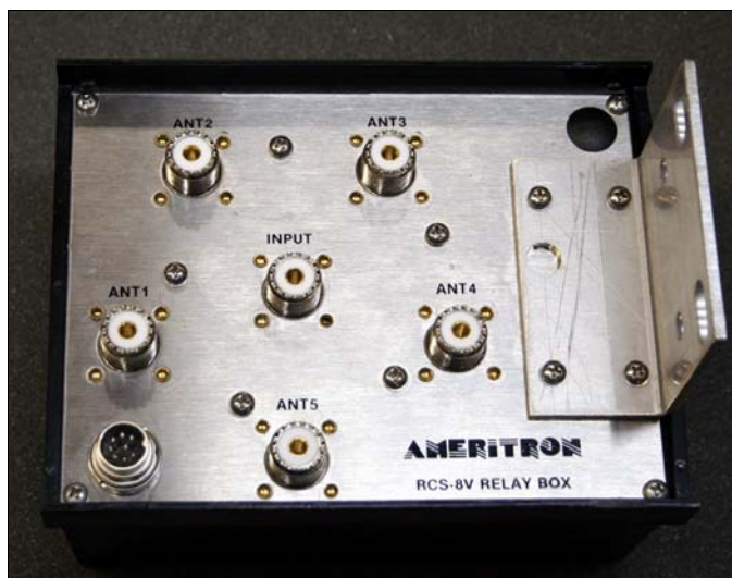
Figure 5 - RCS-8V with Added Interface Connector
