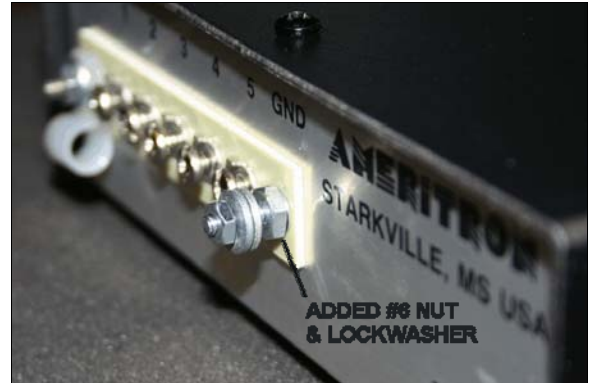
Figure 4 - Improved Ground Terminal
