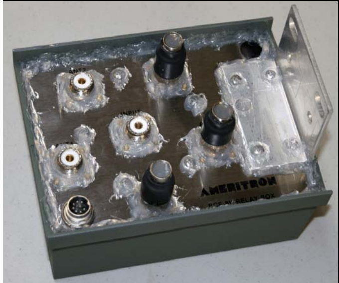
Figure 8 - Completed RCS-8V (Modified, Painted, and Sealed)
